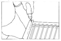
Step 9 - Check overall width is 2.42m. Secure second post as in step 7. Turn panel over and screw in reverse side. Panel is now ready for installation.
