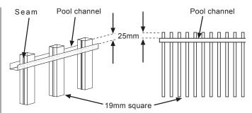
Step 5 - Flip the panel over and tap the pool channel down as in step 4.
