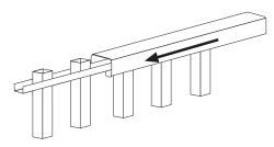
Step 7 - Push the posts over rail by gently squeezing the rail together.
